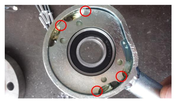
Special care need to be taken during machine pressing. Machine Press Stamp and Support need to have good contact to the whole surface (see next scetch).
