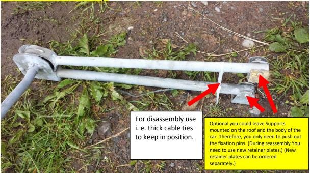
Disassembly of mechanical Components of the Lifting Roof (cable ties (or similar things could help to keep the tension of the springs)
