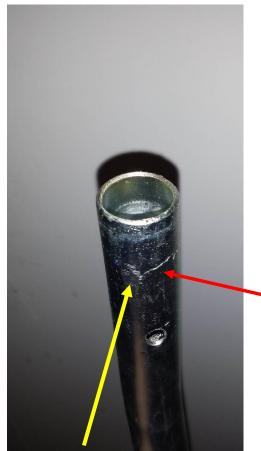
The horizontal Pole can be lightly greased before mounted in the Bearing. Attention: Leftover Grease needs to be removed (cleaned) after assembly in order to prevent stains on the Tent Roof. The welded Pole need to be machined to fit exactly into the Bearing
